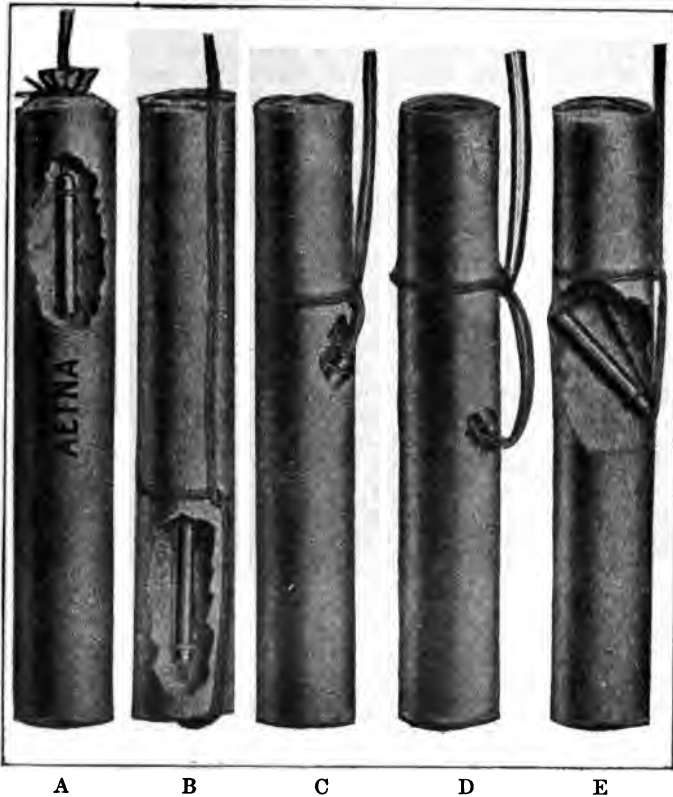
Fig. 91. Different Methods of Inserting an Electric Detonator (Aetna).
